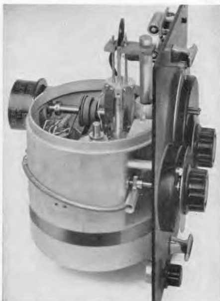
Figure 4. Interior view of the oscillator unit with shield cover removed.
