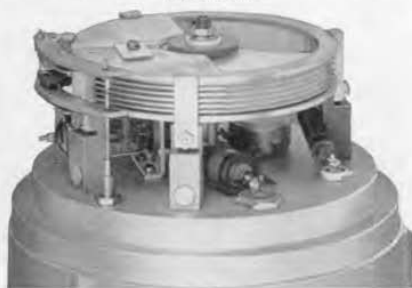
Figure 2. Interior view, showing the location of the two padding capacitors, which are switched into circuit for the 40- to 50-megacycle range extension.
